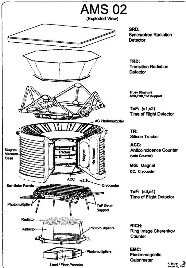
FIGURE 1. View of AMS-02 showing the subdetector components.
