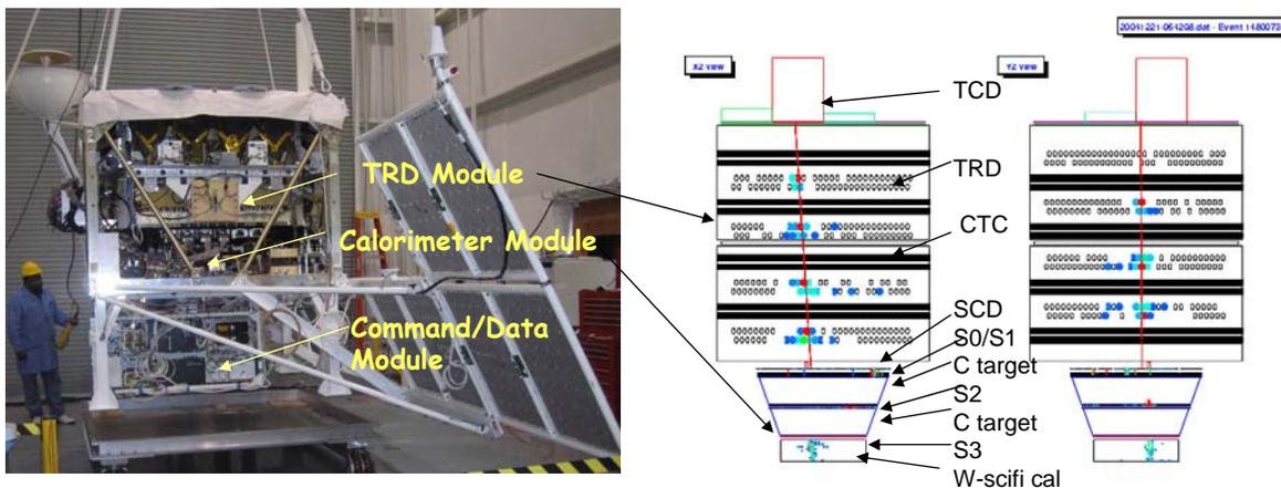
Figure 2. A cosmic-ray Fe nucleus with estimated energy 10 TeV entered the instrument to give a large signal (red box at the top) in the TCD, a clear track in the TRD (blue and red filled circles), a large signal in the SCD (red box) and a well-defined shower in the calorimeter (blue).
