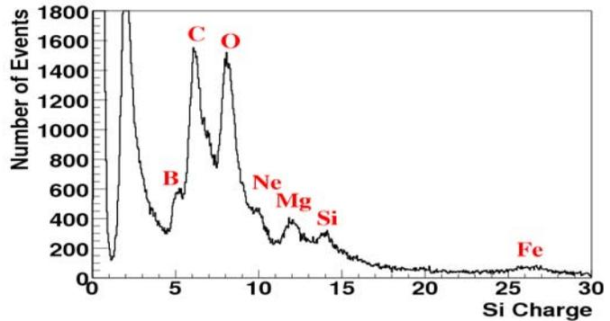
Figure 3. Preliminary flight data: SCD charge histogram without corrections
