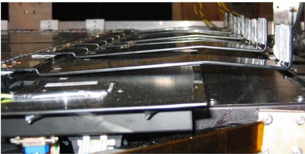
Fig. 4. Part of the copper straps attached at a side of the top cover to conduct out the heat generated in the electronics. A total of 28 straps is connected to the CREAM payload frame from all sides of the SCD cover.
