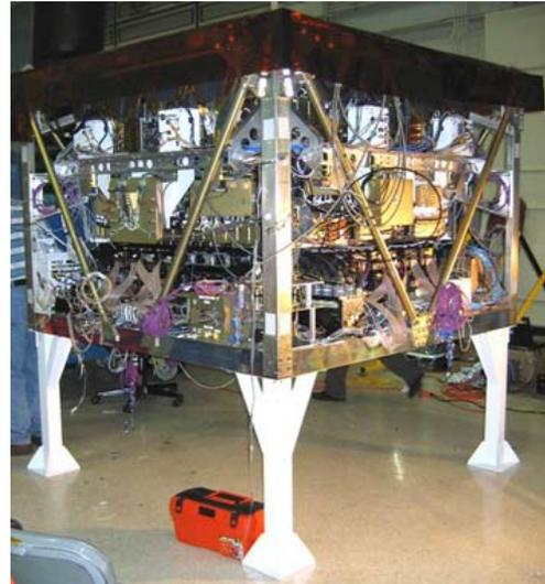
Fig. 5. The CREAM instrument integrated for the environmental test at NASA-GSFC.
