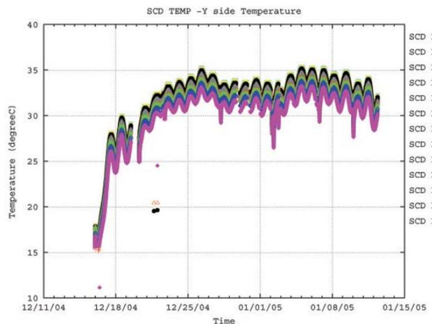
Fig. 6. Variation in the SCD temperature during the flight measured at the front-end analog boards in a side of the detector. The rise in the beginning of the period is the launch fly.
