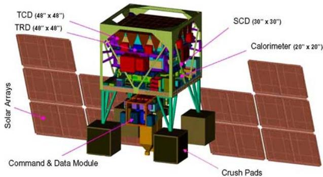
Fig. 1. The CREAM payload and the components.
