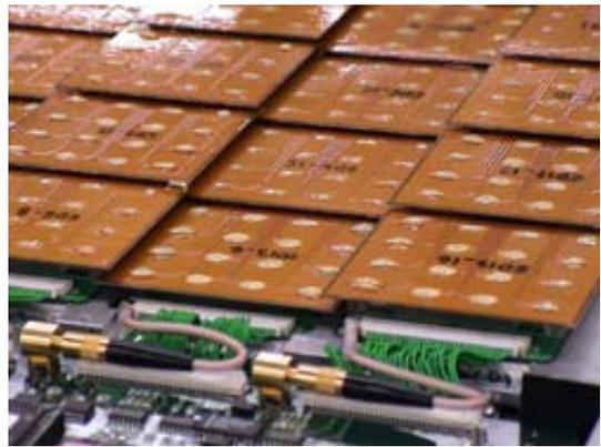
Fig. 2. Part of the SCD assembly. Silicon sensors are arranged with overlapping edges to be dead-region free in all directions. The front-end analog board is installed under the sensors.
