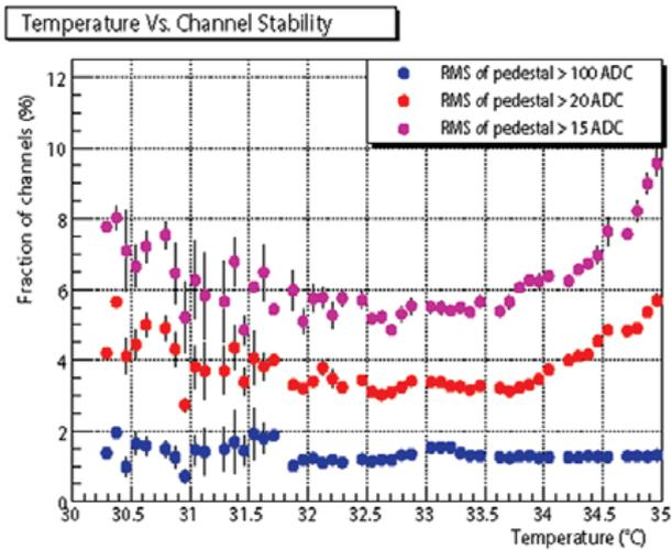
Fig. 3. Fraction of noisy channels vs. detector temperature in the thermal-vacuum test taken before the flight. A noisy channel is defined as a channel with high RMS values of the pedestal signals.
