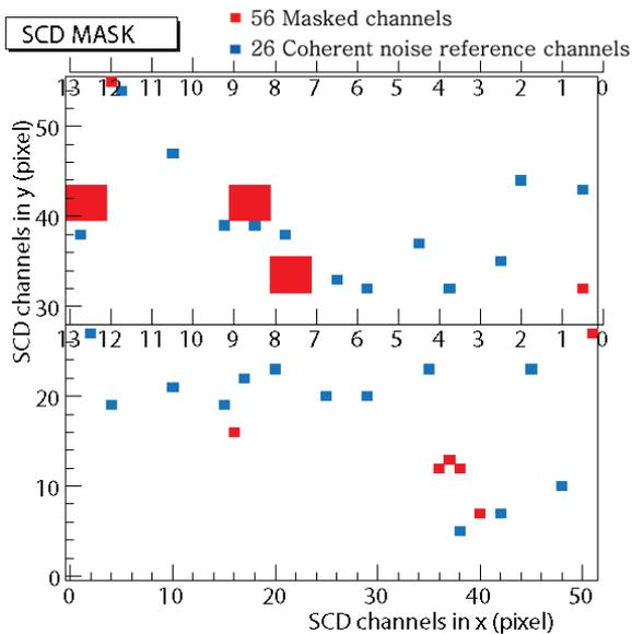
Fig. 7. Bad channel map showing the SCD pixels that were masked during the flight because they were too noisy or dead. Among  $52 \times 56$  SCD pixels, a total of 56 channels were masked (shown in red). The blue spots are 26 channels selected to provide reference data to correct for coherent electronic noise. Their signals were recorded continuously.
