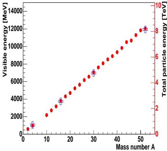
Figure 5. Total visible energy in the calorimeter (left scale) and total particle energy (right scale) for heavy ion fragments versus mass number  $A$  (data : filled circles; simulation : cross markers).
