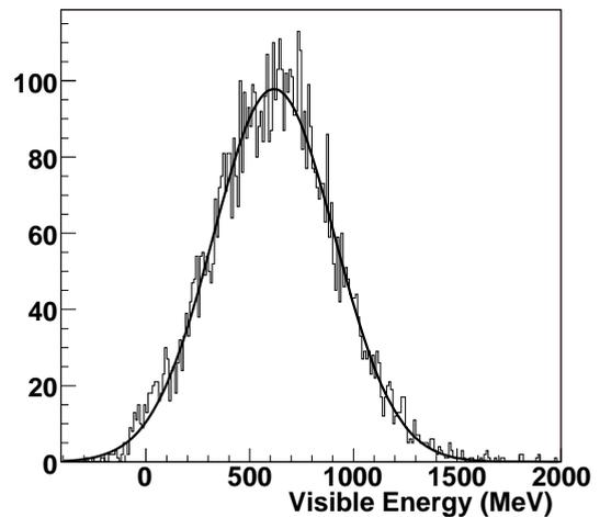
Figure 1. Total visible energy in the calorimeter for 350 GeV protons interacting in the target.
