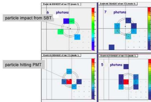
Fig. 4. Examples of events obtained during test beam at CERN in October 2006, with electrons.
