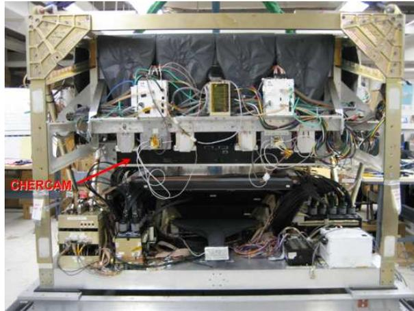
Fig. 6. *CHERCAM instrument integrated.*
