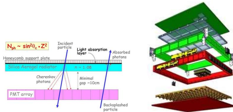
Fig. 2. Scheme of the Cherenkov imager principle (l.h.s.) and . CHERCAM mechanical structure.
