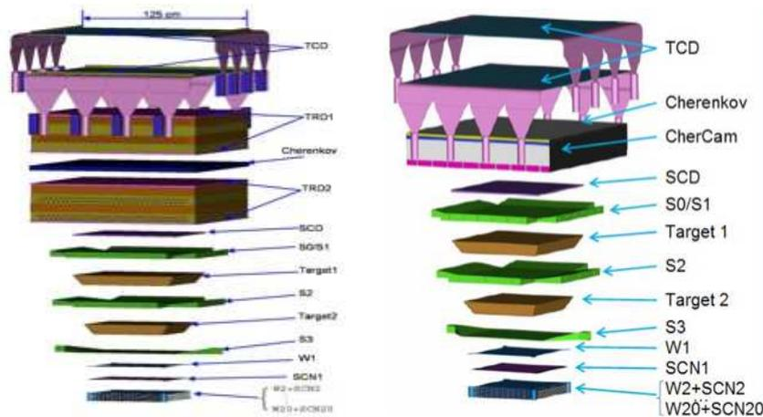
Fig. 1. Exploded view of CREAM instrument, for the 2005 flight (l.h.s.) and the coming one (r.h.s.). This latter includes the CHERCAM imager.
