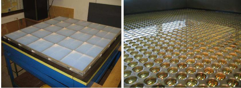
Fig. 3. Chercam aerogel plane (200 tiles, 10x10x105mm) (l.h.s.) and detection plane, made of 1600 PMTs. (r.h.s.)
