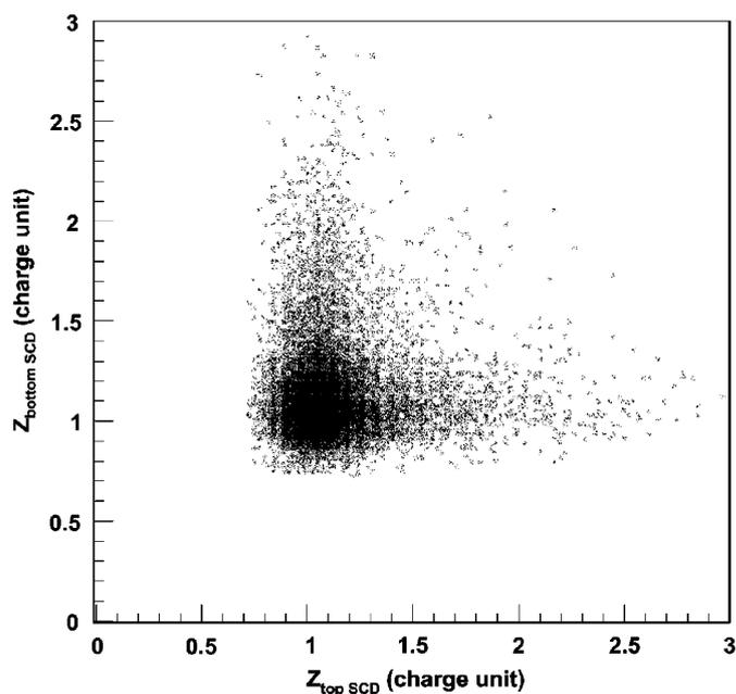
Fig. 4. Signal comparison between top SCD and bottom SCD (signals with value higher than the pedestal mean value +3 sigma were selected in each layer).
