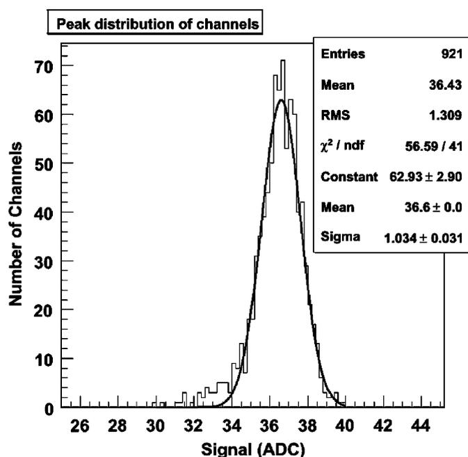
Fig. 3. Peak distribution of channels in the SCD. Peak value was defined by the MPV of the fitted curve.
