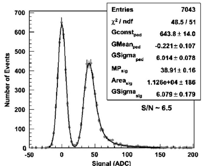
Fig. 2. Signal from one pixel sensor (in top SCD).
