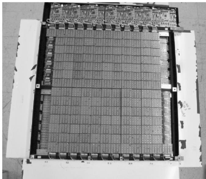
Fig. 1. Dual layer SCD after recovery. Nearly all parts were recovered without damage.
