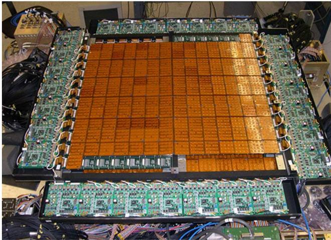
Fig. 3. Fully assembled dual layer SCD for CREAM-II flight. Total 312 sensors (a total of 4992 silicon pixels) shown in the central square are mounted on top of 48 analog boards. 24 digital boards are installed in four rectangular side wings. The top layer is parallel to the bottom one, but rotated about its central point by 90 degrees.
