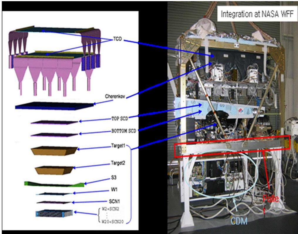
Fig. 1. Component detectors in the CREAM-II payload. The photo was taken in the middle of payload integration at the NASA Wollapse Flight Facility (WFF).
