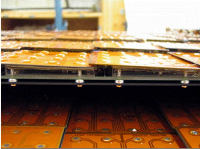
Fig. 2. Assembly of sensors, analog board, and thermal strap.
