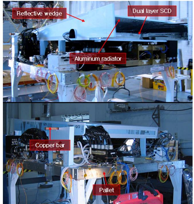
Fig. 4. Reflective wedge installed over the top of the SCD viewed from (a) sun side and (b) anti-sun side. The payload orientation was maintained in flight to keep the solar arrays pointed at the sun, and the radiative wedge opening away from it.
