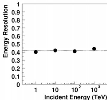
Figure 4. Monte Carlo simulations. The energy resolution, width (1 sigma) of the energy deposit distribution, as a function of the incident energy.
