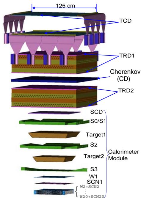
Figure 1. Schematic of the CREAM instrument.
