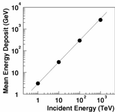
Figure 3. Monte Carlo simulations. Mean energy deposit in the calorimeter as a function of the incident energy.
