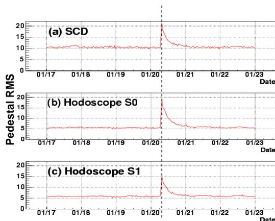
Figure 7. Sudden increase in readout levels during pedestal runs occurred at about 7 am on Jan 20 (GMT) coinciding with a reported powerful solar flare.
