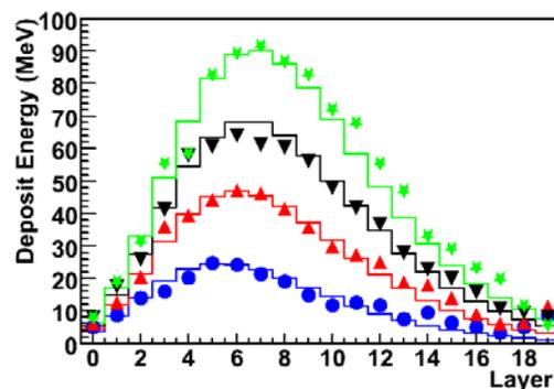
Figure 2. Longitudinal shower profiles for electrons with 50 (blue circles), 100 (red upward triangles), 150 (black downward triangles) and 200 (green star symbol) GeV energies are compared with the Monte Carlo simulations (curves for 50, 100, 150 and 200 GeV from the bottom to top).
