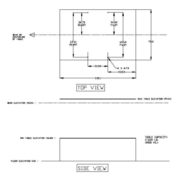
Figure 1. Table Range of Motion and Beam Height
